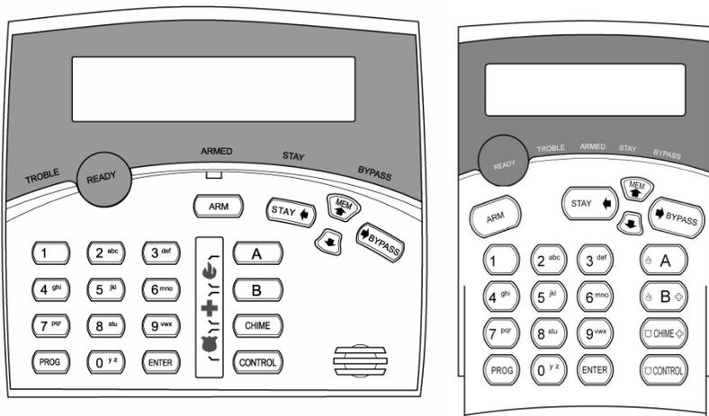
Figure 1: LCD Keypads (Large / Small)
