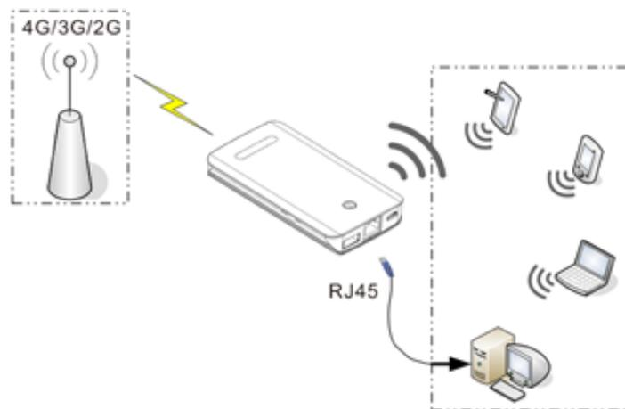
Mode 2 : Inserting Ethernet cable to MIFI-4G RJ45 WAN port to get the internet , and then the terminal devices connect to MIFI-4G by Wi-Fi .
