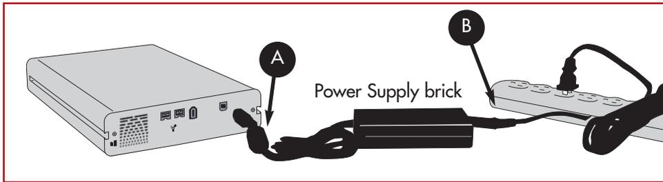
There are two cables that are supplied with the power supply: one cable (A) connects to the LaCie drive; and the other cable (B) connects to a power outlet, such as a wall outlet or a surge protector.
