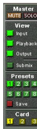
Up to three Firefaces can be used simultaneously. The **Card** buttons switch between the cards. Holding down Ctrl while clicking on button Card2 will open a second window, instead of replacing the current window content.
