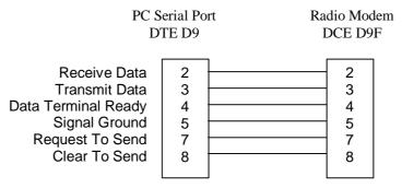
PC connector (9 way) to radio modem (9 way)
