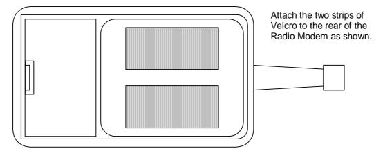
Placement of the adhesive Velcro on the rear of the radio modem.
