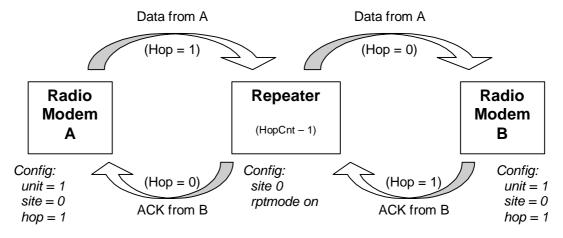
Point-to-point link showing data and return ACK path with their respective hop counts for traversing the repeater.
