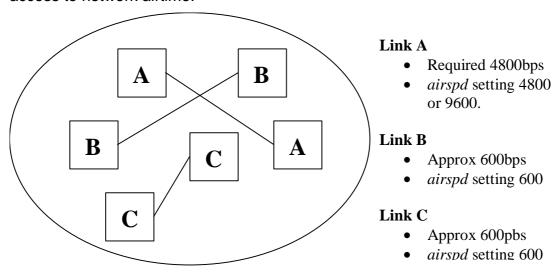
Example network of point-to-point links operating within close radio proximity using different airspeed settings
