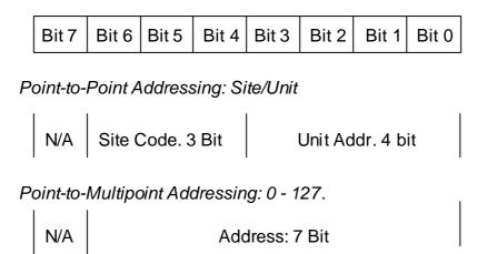
In its most basic form the site code and unit address combined allow up to 127 unique point-to-point link paths. That is to say that up to 127 point-to-point links may operate successfully (but not necessarily at maximum through put rate) within close radio proximity to one another.
