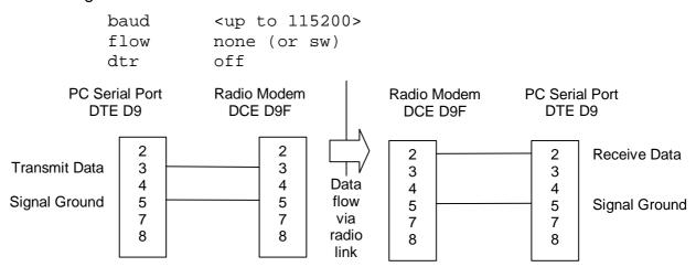
Two wire simplex connection to the radio modem.
