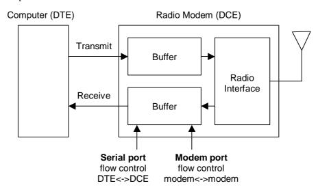
Two kinds of radio modem flow control - Serial port and Modem port
