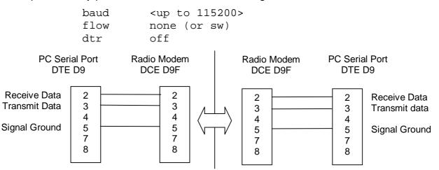
Three wire half duplex connection to the radio modem
