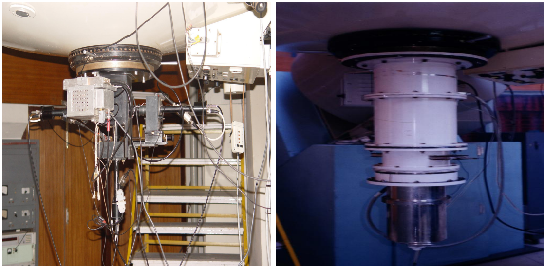
Figure 3.4: Photographs of the Fast photometer and Imaging polarimeter as mounted at the Cassegrain end of the telescope.
