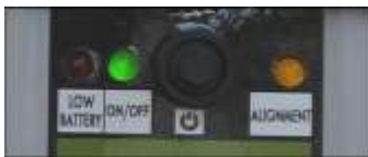
Fig. 14: Receiver & Beam Emitter are aligned. The Alignment LED is ON.
