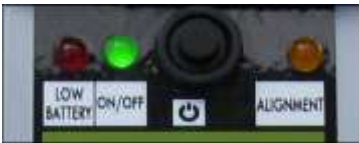
Fig. 13: a) Unit is ON – Alignment LED is OFF, indicates that the receiver is not able to "see" the Emitter
