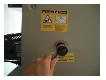
When removing the jam, turn the press rollers by inserting the jam removal ratchet and turn it clockwise like the picture.
