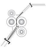
4. The form hits the lower cassette stopper and forms a buckle. The folded form then enters in between the two outer rollers.
