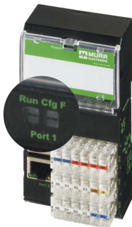
Fig. 15: Run LED on the Cube20 PNIO DI8 Art. No. 56006
