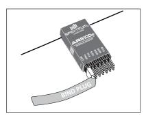
Power on the receiver. If the receiver is installed in an electric aircraft, turn on the speed controller to power up the receiver. If the receiver is going to be powered by a separate battery, plug the battery into any unused port. The amber light will blink, indicating the AR6100E is in bind mode.
