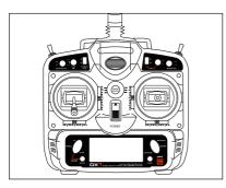
Press and hold the bind button on the back of the transmitter while turning on the transmitter. The button will flash for several seconds, then the LED on the transmitter and receiver will remain solid on, indicating a successful bind.
