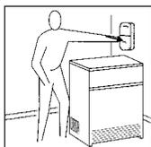
**7** The electrical isolator switch must be within hand reach of the installed machine.
