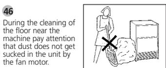
During the cleaning of the floor near the machine pay attention that dust does not get sucked in the unit by the fan motor.
