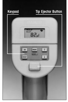
There are six EDP2 models. Each model is completely adjustable within its range: the smallest settable volume increment is  $0.02\mu L$  for the Micro-10 EDP2, 1/500 of full range for 100 and 1000 $\mu L$  models, and 1 /250 of full range for 25, 250, and 2500 $\mu L$  models.
