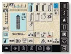
**Customised Buttonholes:** As well as on-screen setting of the buttonhole length, the slit width can also be changed – from 0.1 to 2 mm – to accommodate any type of button you may be using. The buttonholes can then be perfectly repeated as often as you wish.
