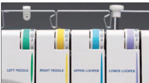
Labeled and numbered tension guides mean no guess work for adjustments. Normal tension settings are all marked.
