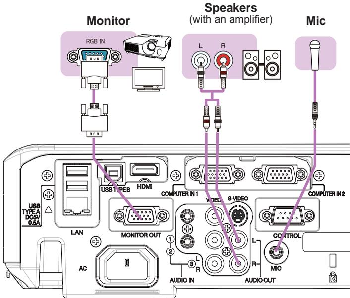
**NOTE** • If a loud feedback noise is produced from the speaker, move the microphone away from the speaker.
