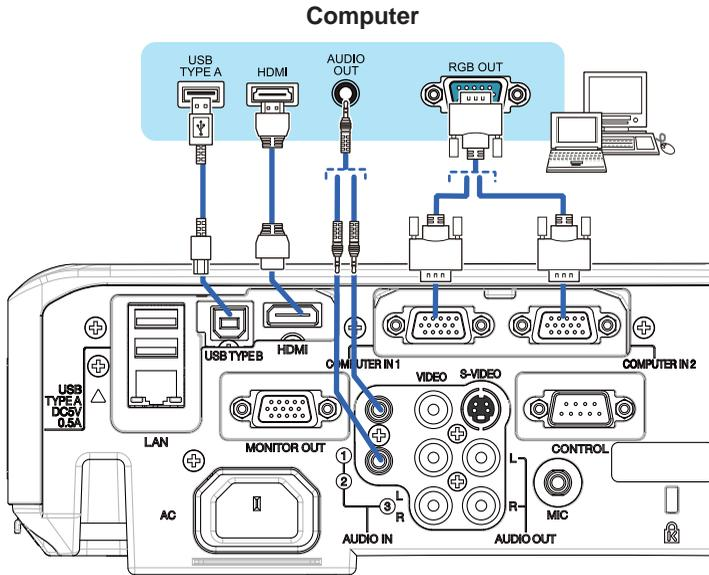
**NOTE** • Before connecting the projector to a computer, consult the computer's manual and check the compatibility of the signal level, the synchronization methods and the display resolution output to the projector.
