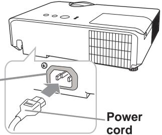
Please remember that when the DIRECT POWER ON function activated (📖 58), the connection of the power supply make the projector turn on.
