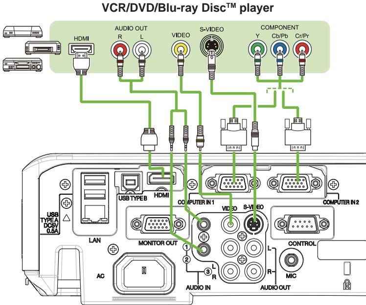
**NOTE** • The **HDMI** port of this model is compatible with HDCP (High-bandwidth Digital Content Protection) and therefore capable of displaying a video signal from HDCP compatible DVD players or the like.
