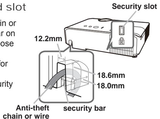
**⚠WARNING** ▶ Do not use the security bar and slot to prevent the projector from falling down, since it is not designed for it.
