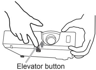
**⚠ CAUTION** ▶ Do not handle the elevator button without holding the projector, since the projector may drop down.
