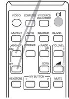
2. The display magnification of the projector switches in order with every press of the **MAGNIFY ON** button.
