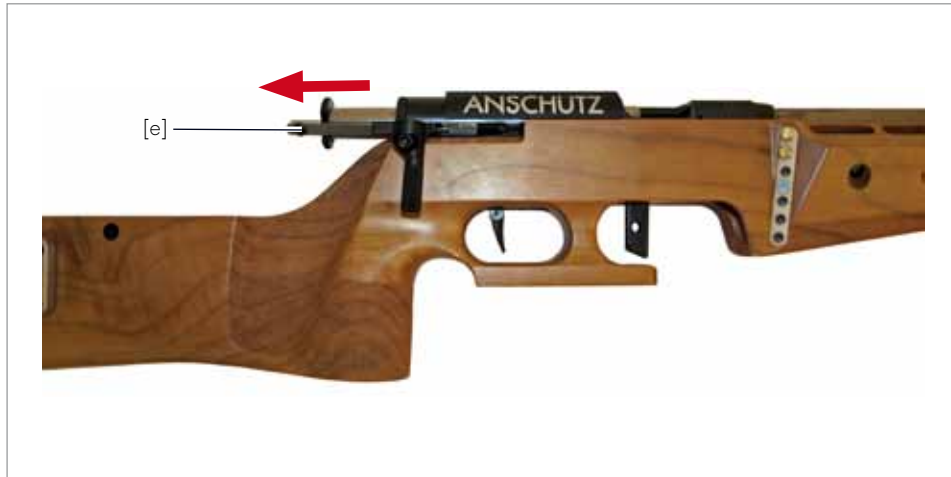
Fig.18 Extracting the breech wedge
