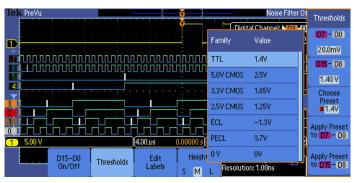
With the color-coded digital waveform display, groups are created by simply placing digital channels together on the screen, allowing the digital channels to be moved as a group. You can set threshold values for each pod of eight channels, enabling support for up to two different logic families.
