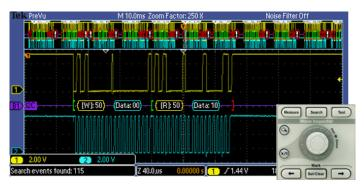
Search – I<sup>2</sup>C decode showing results from a Wave Inspector search for Address value 50. Wave Inspector controls provide unprecedented efficiency in viewing and navigating waveform data.
