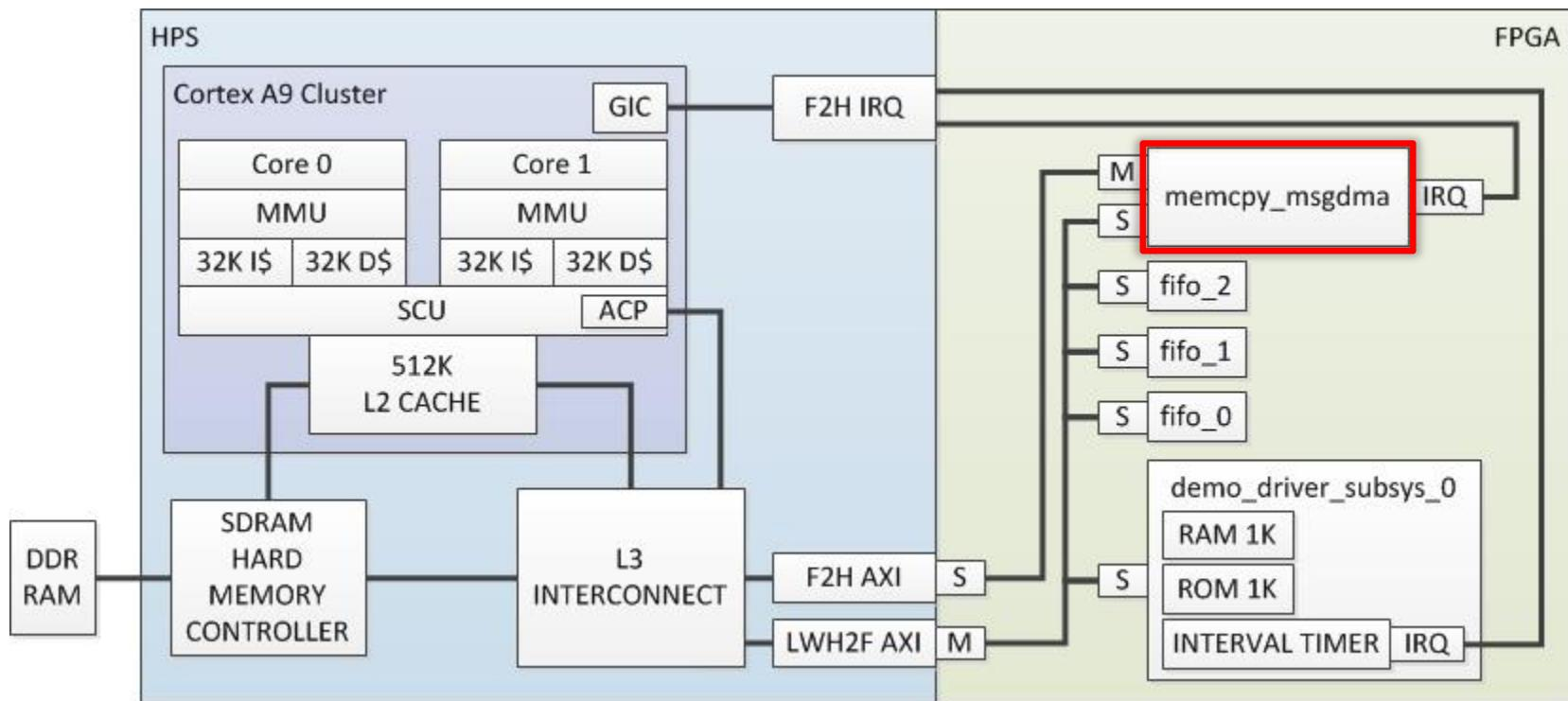
The **memcpy\_msgdma** component can be used to DMA data thru the F2H AXI bridge, which allows us to DMA data to/from anywhere in the HPS core or peripherals attached to the LWH2F and H2F AXI bridges in the FPGA.
