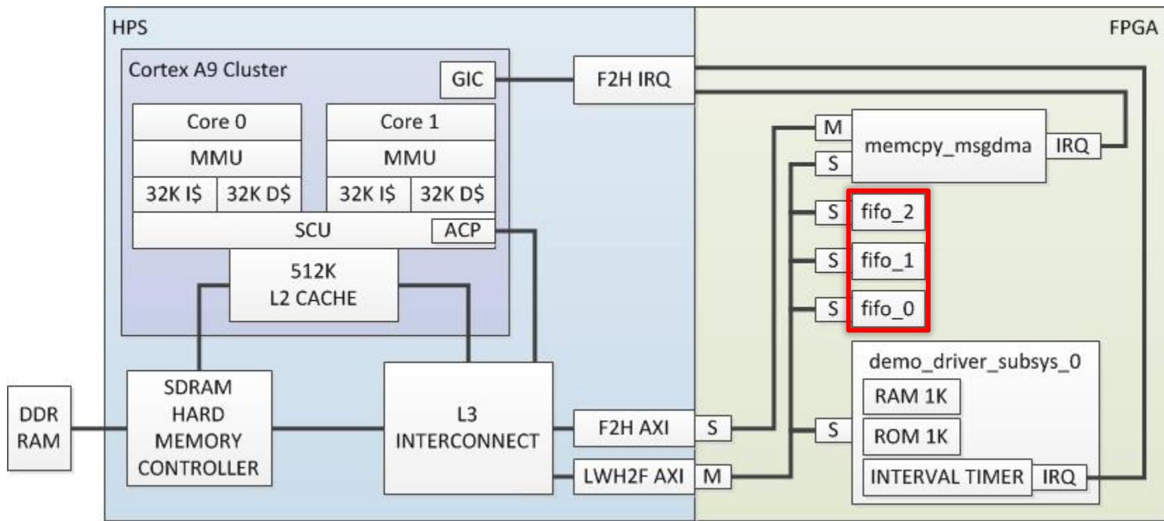
There are three FIFO components that have a slave interface for writing data into the FIFO and another slave interface for reading data out of the FIFO. In this block diagram the FIFO is represented with only one slave interface for simplicity.
