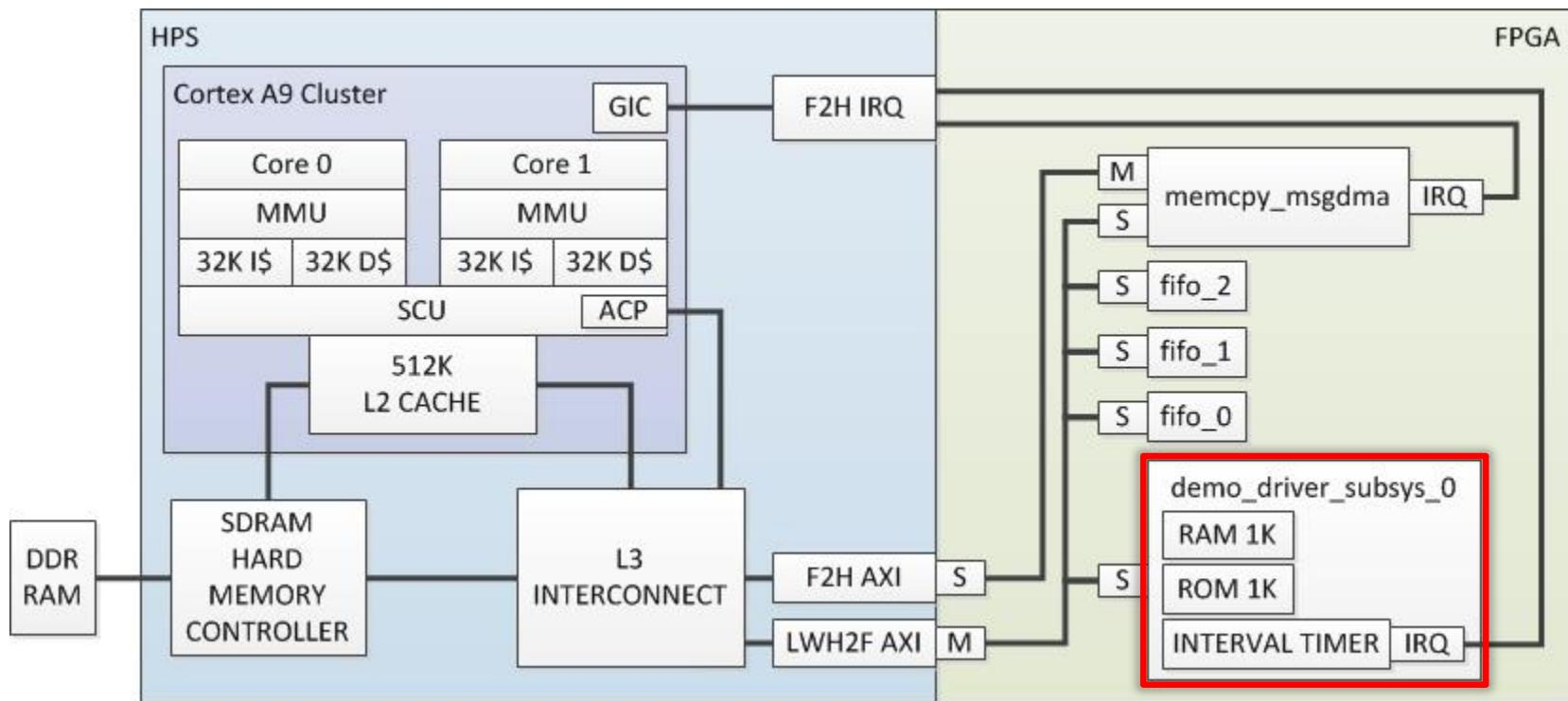
The **demo\_driver\_subsys\_0** peripheral is a custom Qsys component that presents one opaque slave interface to the system. Internally it contains a RAM, a ROM, and an Interval Timer that can generate an interrupt.
