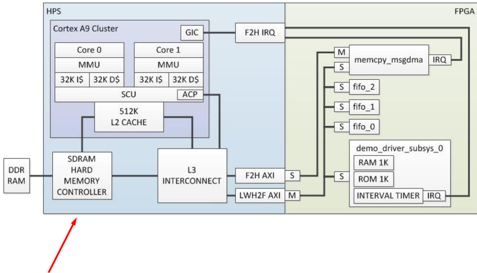
This is a very simplified block diagram of the Altera HPS and FPGA system that is used to demonstrate the concepts described in this workshop. Please see the Qsys system for more detail.
