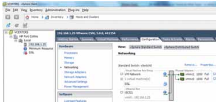
Figure 1 – Standard Virtual Switch – Two Physical Adapters
