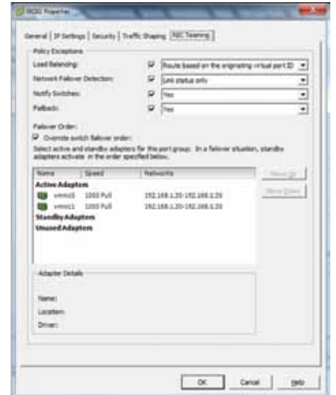
Figure 2 – iSCSI VMkernel Properties – NIC Teaming
