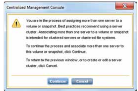
Figure 18 – Assigning multiple servers to a single volume
