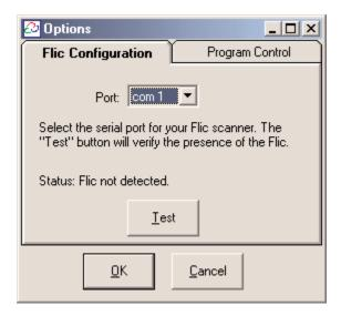
If, after pressing the Test button, the status line says, "Flic not detected," check the connections, and/or try another port.
