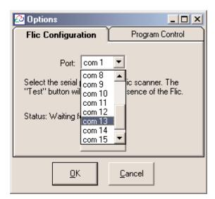
If the Flic is not detected, check the cable connections. If the cable is connected properly, try using other ports.
