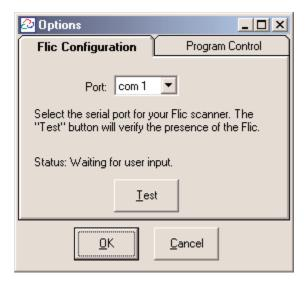
When this window launches, you'll notice that the message area of the Options window says, "Status: Waiting for user input." Ensure that the Flic scanner is attached to its cable, and that the cable is attached to an RS-232 port on your computer. Select the port's ID, and press the Test button.
