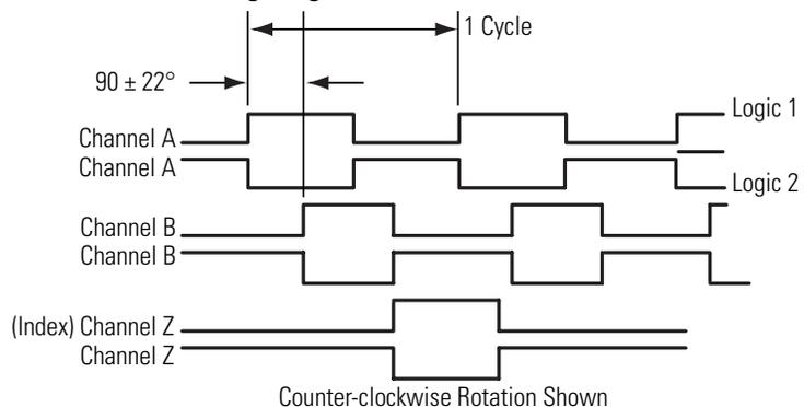
2. Look at the Z input signal and its complement Z signal on the timing diagram. Whichever signal is low for most of the encoder revolution and pulses high for the marker interval should be wired into the Z(+) terminal. The remaining signal should be wired into the Z(-) terminal.
