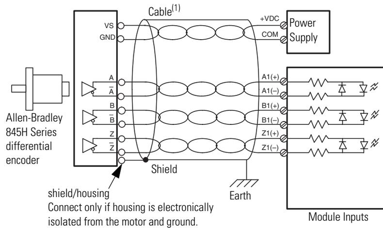
(1) Refer to your encoder manual for proper cable type. The type of cable used should be twisted pair, individually shielded cable with a maximum length of 300m (1000 ft.).
