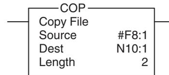
The source is the floating-point file, and the destination is an integer data file. The length is 2, the number of elements being copied into the destination file using the copy instruction.
