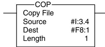
The source is the input data file, and the destination is the floating point file. The length is 1, the number of elements of the destination file in the COP instruction.
