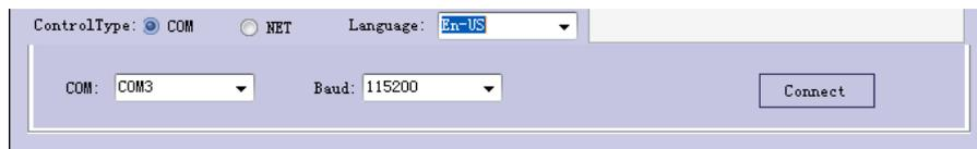
Figure 4.3 Serial port connection
