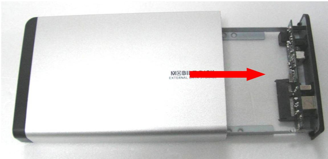
**STEP2:** Push the Hard Drive toward the SATA connector and make sure the SATA connector is properly connected.
