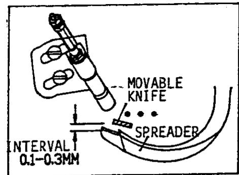
WHEN MOVEABLE KNIFE MOVE FORWARD AND MEET WITH SPREADER, THE TIP OF HOOK BLADE SHOULD SQUARE MATCH TO THE THREAD HOOK OF SPREADER. LOOSEN THE SET SCREW, ADJUST THE HOOK BLADE OF MOVABLE KNIFE TO ITS PROPER POSITION AND LINE UP WITH THREAD HOOK OF SPREADER THEN TIGHTEN THE SET SCREW.
