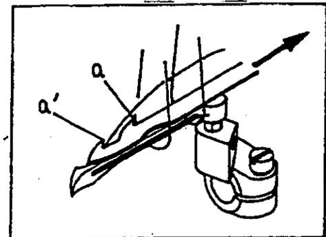
THE TRIMMING ABILITY OF KNIFE MUST BE MODERATE OR THE KNIFE WILL BE WORN OUT VERY SOON. IF THE TENSION OF KNIFE PRESSURE SPRING IS TOO BIG, YOU CAN ADJUST IT BY MOVING KNIFE PRESSURE SPRING TO THE RIGHT OR LEFT IN ORDER TO GET PROPER TENSION.
