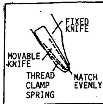
ADJUSTING SCREW IS USED FOR SETTING THE TENSION OF CLAMP SPRING IN ORDER TO HOLD THE ORNAMENTAL THREAD PROPERLY. IF THE TENSION BETWEEN THREAD CLAMP SPRING AND MOVABLE KNIFE IS TOO BIG, THEN MOVE THE KNIFE PRESSURE SPRING FORWARD IN ORDER TO GET PROPER TENSION.
