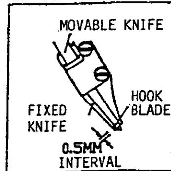
WHEN MOVABLE KNIFE MOVE TO ITS UPPERMOST DEAD POINT, THE FRONT EDGE OF THREAD CLAMP SPRING AND MOVABLE KNIFE SHOULD BE EVEN. AND THE FRONT EDGE OF KNIFE PRESSURE SPRING AND FIXED KNIFE SHOULD BE EVEN.
