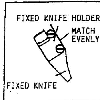
WHEN MOVABLE KNIFE MOVE BACKWARD, THE HOOK BLADE OF MOVABLE KNIFE SHOULD RETREAT 0.5m.m. INSIDE FROM THE BLADE OF FIXED KNIFE.
