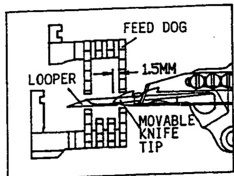
WHEN MOVABLE KNIFE KEEP MOVING TO THE LEFT TILL 1.5mm AWAY FROM THE RIGHT SIDE OF FEED DOG'S LEFT COLUMN. THE TIP OF THE MOVABLE KNIFE SHOULD STILL STAY WITHIN THE RIDGE OF THE LOOPER.
