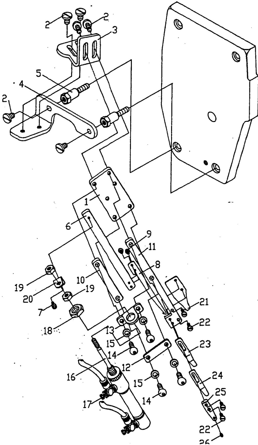
Spreader Thread Trimmer Components (FOR 756U MACHINES)
