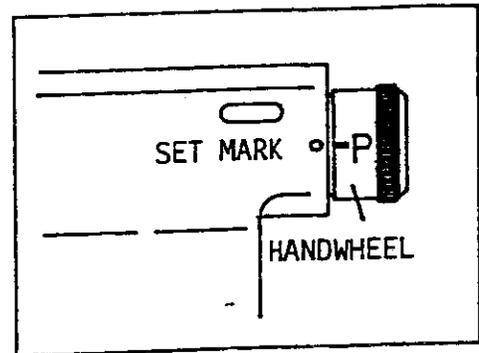
KEEP PUSHING THE PISTON OF KNIFE DRIVING CYLINDER, THEN THE MOVABLE KNIFE START TO MOVE FORWARD.
