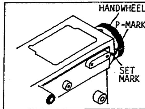
1. INSTALL SYNCHRONIZER ① INTO BELT PULLEY ③ AND TIGHTEN THE SET SCREW ② LIGHTLY.
