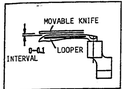
LOOSENING THE SET SCREW A AND ADJUSTING THE HEIGHT OF LOWER FIXED KNIFE CARRIER GUIDE TO ITS PROPER POSITION THEN TIGHTEN THE SET SCREW A. PLEASE MAKE SURE THE LOWER MOVABLE KNIFE CAN BE MOVED FORWARD AND BACKWARD SMOOTHLY.
