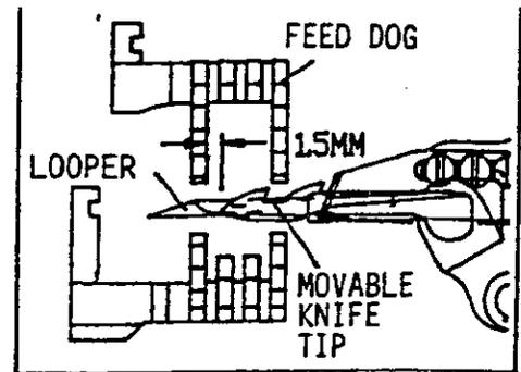
WHEN ADJUSTING, LOOSENING THE SET SCREW (A) AND TURNING THE ECCENTRIC STUD AND SETTING THE POSITION OF THE TIP OF MOVABLE KNIFE (THE SET MARK OF THE ECCENTRIC STUD MUST FACING TOWARD THE RIGHT SIDE).
