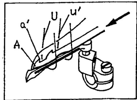
WHEN MOVABLE KNIFE (A) RETREAT FROM ITS LEFTTEST DEAD POINT TO THE RIGHT, HOOK BLADE (a) AND (a') WILL PULL THE NEEDLE THREAD AND LOOPER THREAD TO THE FIXED KNIFE AND CUT THE THREADS IN ORDER AND THE CLAMP SPRING WILL HOLD THE THREAD END AND MOVE TO THE BACK OF LOOPER TOGETHER WITH TRIMMING KNIFE SET (A). YOU CAN ADJUST THE HOLDING PRESSURE OF CLAMP SPRING TO AVOID THE THREAD END CAME OFF DURING THE MOVEMENT BY ADJUST CLAMP SPRING PRESSURE ADJUSTING PIECE.
