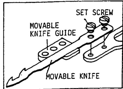
WHEN MOVABLE KNIFE MOVED TO ITS LEFTTEST DEAD POINT THERE SHOULD HAVE A INTERVAL OF 1m.m. BETWEEN SET SCREW A AND FIXED KNIFE AND CAN NOT COLLIDE WITH EACH OTHER. YOU CAN ADJUST THE INTERNAL BY LOOSEN THE SET SCREW B AND MAKE SURE THE EDGE OF MOVABLE KNIFE MATCH EVENLY WITH THE EDGE OF FIXED KNIFE.
