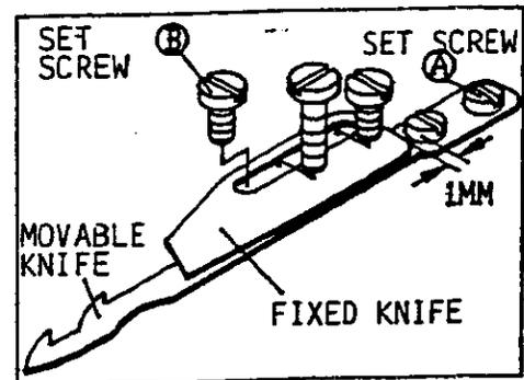
WHEN MOVABLE KNIFE MOVED TO ITS RIGHTTEST DEAD POINT, THE HOOK BALDE OF MOVABLE KNIFE SHOULD BE RETREAT 1m.m. INSIDE FROM THE BLADE OF FIXED KNIFE.
