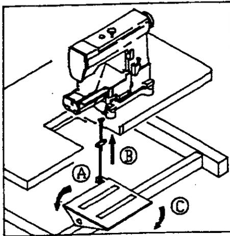
1. START THE SEWING MACHINE BY PUSHING THE PADEL FORWARD (A)
