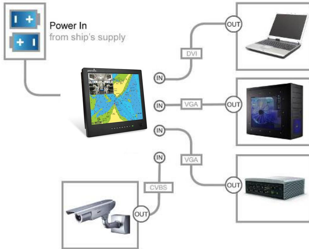
Remarks: The real installation diagram above is only for reference and will differ for different kinds of applications.
