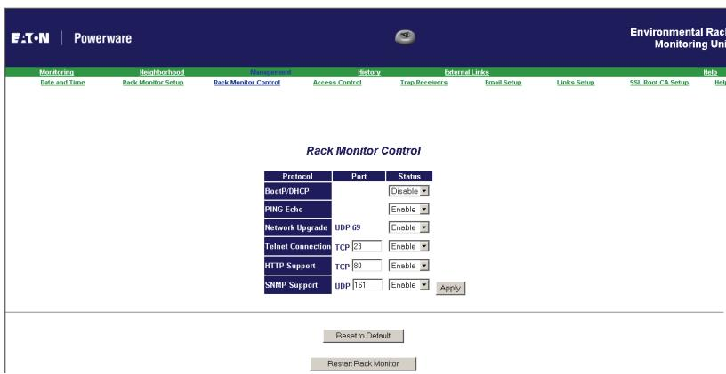
**Figure 21. Rack Monitor Control Screen**
