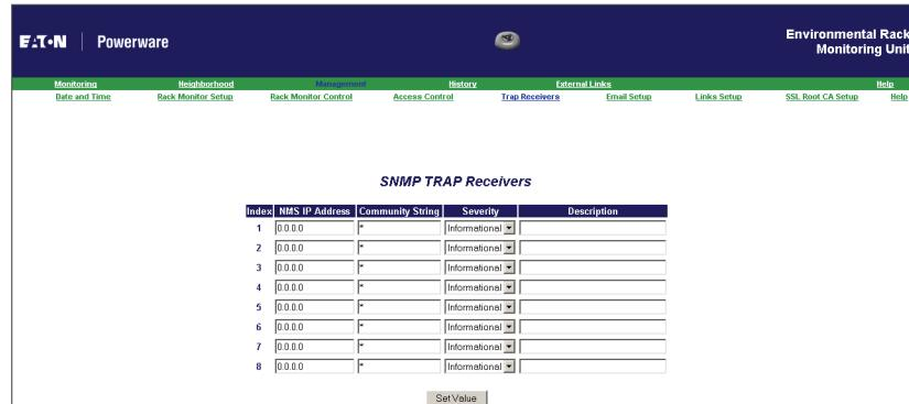
**Figure 32. SNMP TRAP Receivers Screen**
