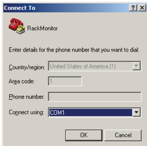
**Figure 6. Select Direct to COM Port Connection**
