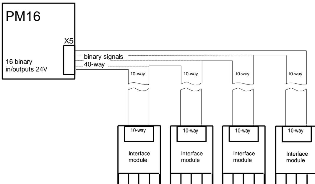
Additional PM16 components:a) Serial Interfaces
