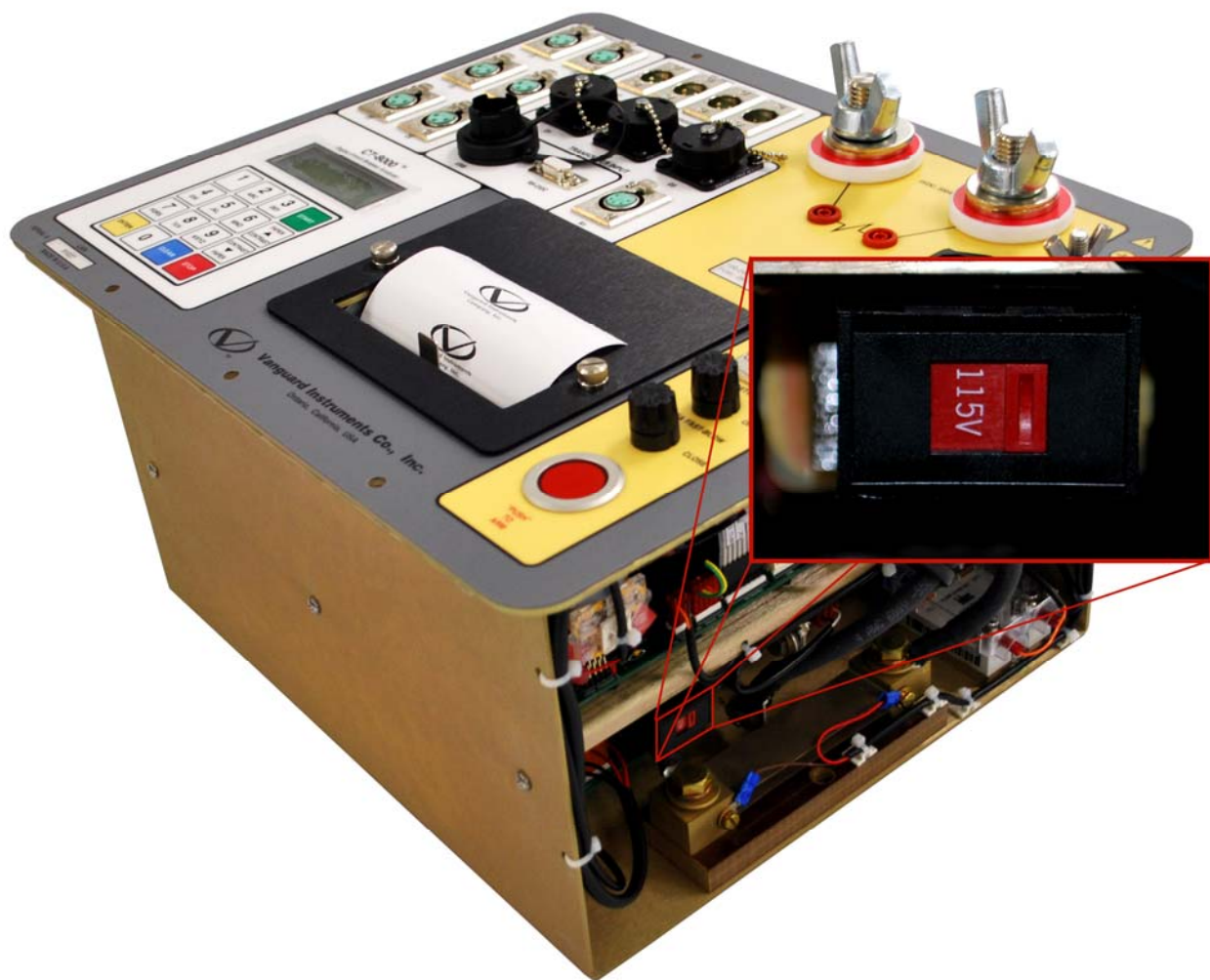
Figure 2. CT-8000 Operating Voltage Setting Switch
