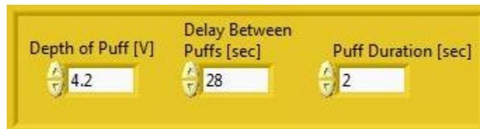
2. For other user-defined protocols, adjust the **Depth of Puff** voltage to between 0-5 V, to achieve a puff volume between 0 and 66 ml (see next section regarding puff volume calibration) for a 2 second puff. To increase the amount of cigarette smoke generated, increase the number of puffs per minute by decreasing the **Delay between Puffs** interval.
