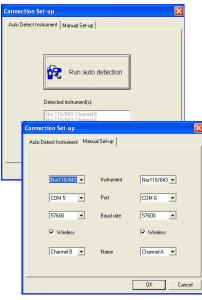
After the scan has finished all detected instruments are listed below the button together with the type and name of instrument. In addition the COM port number, baud rate and type of connection are set up according to the result of the auto detection.
