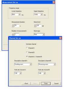
four measurement modes *Level*, *Reverberation*, *Background* or *Impact*. All that is required then is to set the measurement parameters and define the channel allocation. The frequency range can be selected
