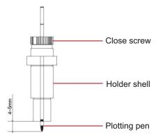
Cutting plotters can be just as easily used as a pen plotter for CAD/CAM work, just insert the pen holder (supplied) and you can use the ball pen as plotting pen; keep the ball pen out of the holder between 4mm to 5mm. (3/16 inch)
