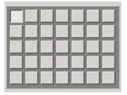
To the right of this is a black grid of rectangles is the <u>Key Data Editor</u>. It holds the data associated with each key on the keypad.
