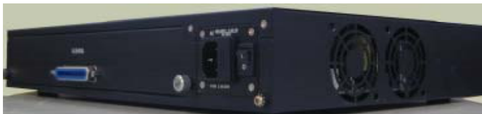
Fig 1-4 SHDSL IP DSLAM Rear View
