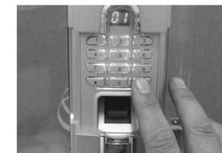
(if you do not complete Step 4 above within 5 seconds, the mode will be changed to main control mode and LED displays “no”).
