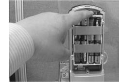
**Step 2:** Pull up the sliding cover in the front body of the lock within 10 seconds upon the completion of Step 1. You should see the fingerprint sensor light up in red
