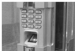
**Step 3:** Place the master finger or the sub-master finger on the glass of the sensor to verify (LED displays “FO-no”)
