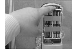
**Step 2:** Pull up sliding cover in front body of the lock
