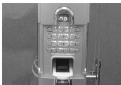
\* “no” in LED means the lock is waiting for entry of function codes (for example : “01” for sub-master or user enrolment) for further programming. (refer to 3.1 for programming code table)
