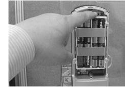
**Step 2:** Pull up the sliding cover in the front body
