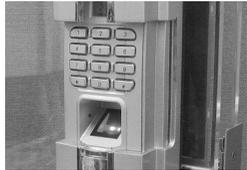
**Step 3:** Place the master finger or the sub-master finger on the glass of the sensor to verify (LED displays “no”)
