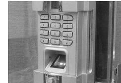
**Step 3:** Place master finger or sub-master finger on the glass of the sensor to verify (LED displays "FO-no")
