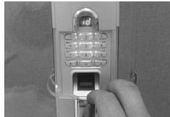
**Step 5:** Enter the ID number (2 or 3 digits) of the enrolled fingerprint you wish to delete and press "#" button. A triple beep sound and a green light indicate the success of the fingerprint deletion.
