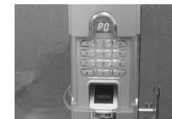
**Step 5:** Press the pincode at ID(01) and "#". Voice prompt saying "Function installed" will be heard to indicate successful total deletion including sub-master fingerprint
