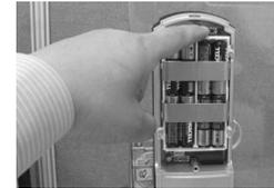
**Step 2:** Pull up the sliding cover in the front body of the lock
