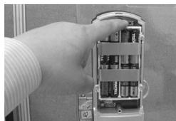
**Step 2:** Pull up the sliding cover in front body of the lock
