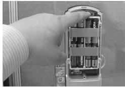
**Step 2:** Pull up the sliding cover in the front body of the lock
