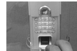
**Step 5:** Enter “0” then press “#” button. Voice prompt saying “Function installed” will be heard to indicate success of automatic sensor on mode setting.
