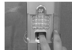
\* A triple beep sound and a green light indicate the success of the sub-master finger enrollment and LED displays "id" for more sub-master finger enrollment.
