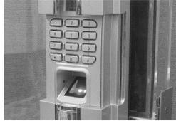
**Step 3:** Place the master finger or the sub-master finger on the glass of the sensor to verify (LED displays "F0-no")
