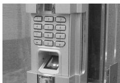
**Step 3:** Place the master finger on the glass of the sensor to verify (LED displays “F0-no”)
