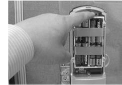
**Step 2:** Pull up the sliding cover in the front body of the lock (The fingerprint sensor will then turn on with a red light)
