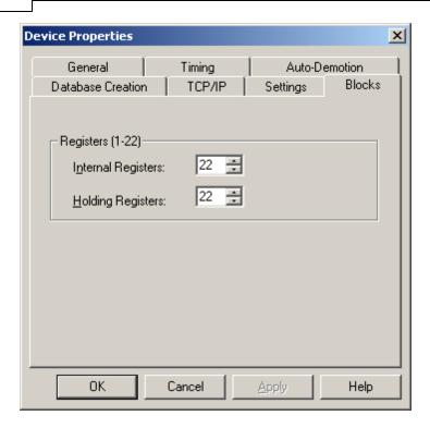
Given the overhead involved in sending data via TCP/IP, it is generally advantageous to keep the block size large. However, if data will be read from non-contiguous locations within the device, reducing the block size may increase performance.
