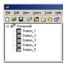
Each device appears under a single Honeywell UDC Ethernet channel. In this configuration, the driver must move from one device to the next as quickly as possible in order to gather information at an effective rate. As more devices are added or more information is requested from a single device, the overall update rate begins to suffer.
