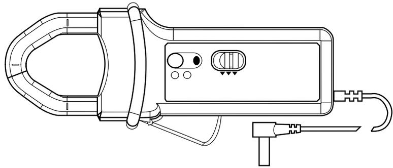
Model PAC11 is a high precision clamp-on current meter that operates using Hall effect technology for the measurement of AC and DC currents. There is a mV output for direct measurement reading on a multimeter, and an automatic DC zeroing system.
