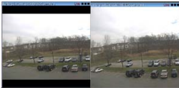
Example: The same image viewed with Maintain Image Aspect Ratio selected (left) and cleared (right)
