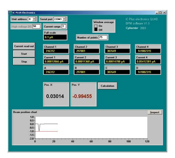
This program allows to control the IC plus Quad in the remote mode by means of the RS232 communication port and performs beam position monitoring.
