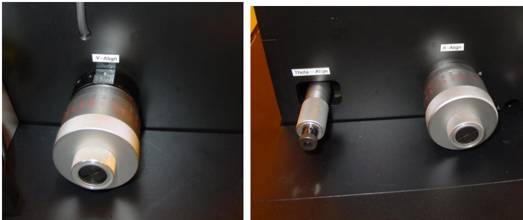
Figure 4. Left side micrometer knob moves the stage in the Y-axis, while the large micrometer on the right side moves the stage in the X-axis. The small micrometer knob on the right side rotates the wafer.
