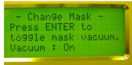
Figure 8. CHANGE MASK display with vacuum toggle note.
