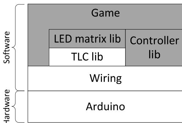
Fig. 7. The architecture of the software
