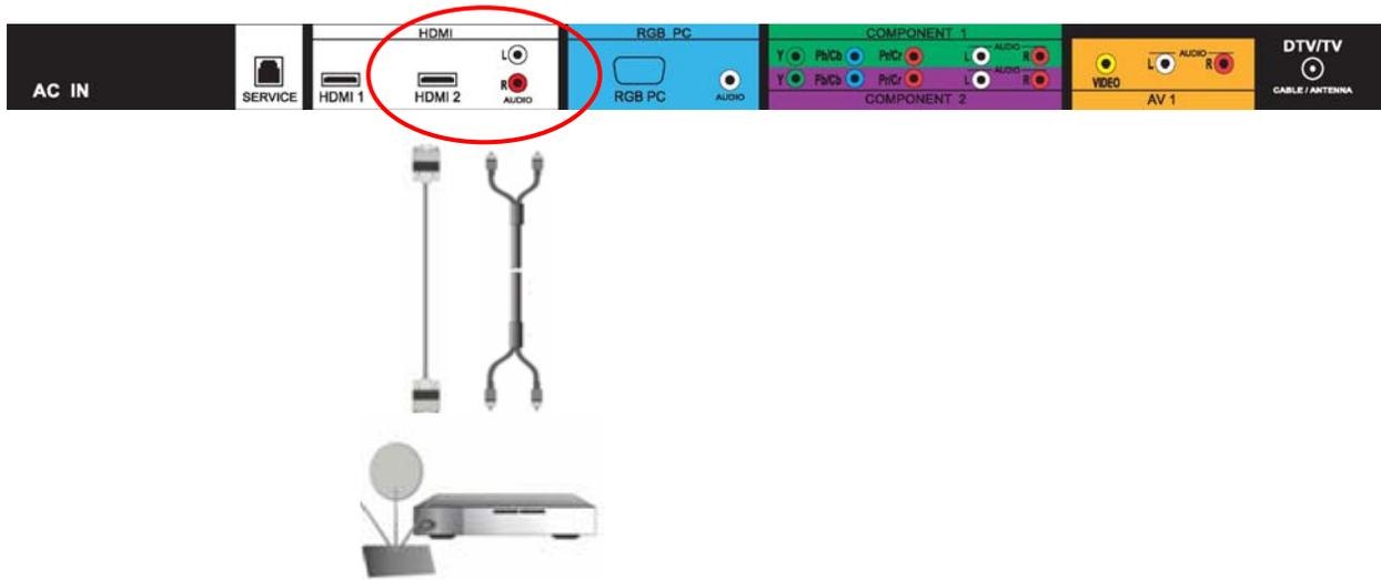
1. Turn off the power to the HDTV and HDTV Set-Top Box.
