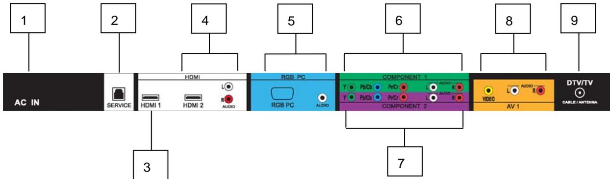
1. **AC IN** – Plug-in the supplied AC Power Cord here.
