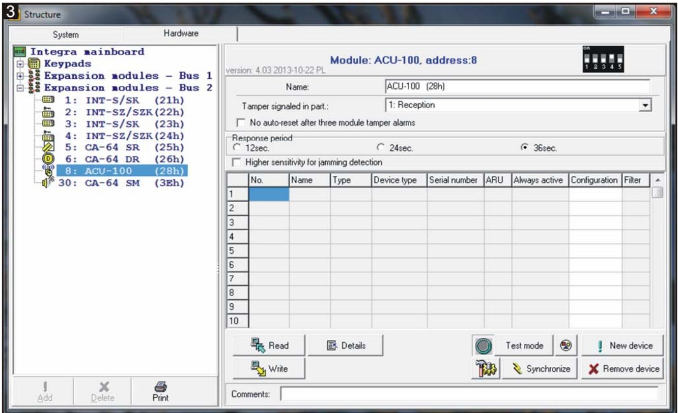
**Higher sensitivity for jamming detection** – if this option is enabled, the sensitivity of detection of radio communication jamming is boosted.
