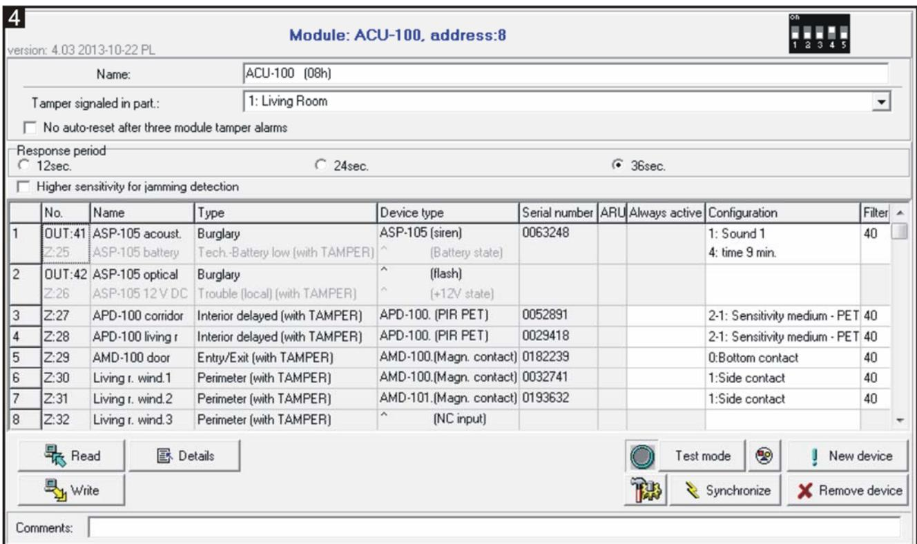
For each group of 8 zones /outputs, one address on the expander bus is reserved. The controller can occupy from 1 to 6 addresses. This must be taken into account at the system design stage and sufficient number of free addresses must be left for the controller. If, when new wireless devices have been added to the controller, it turns out that next addresses are needed, and these are taken up by other devices, successful completion of the expander
