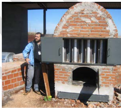
Image 21: Furnace for combustion of biogas
