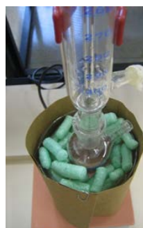
Image 7: fermenter on top of the heating system
