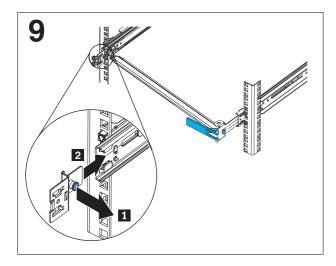
Install the cable management arm mounting bracket.
