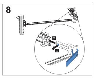
Install the cable management arm stop bracket.
