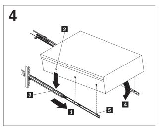
Install the server on the slide rails.
