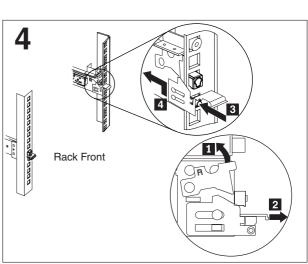
Remove the rear end of the slide rails.
