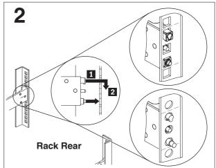
**Install the rear end of the slide rails. Note:** When you install a 4U server, be sure to install the slide rails in the second U from the bottom of the 4U area in the rack.
