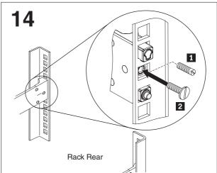
Install the front screws, if necessary.
