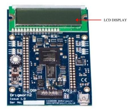
The standard Drigmorn2 LCD display is an LCM-S01602DTR/M display, which is 16x2 alpha-numerical display with a Hitachi HD44780 compatible chipset. More information on this at <a href="http://www.lumex.com/specs/LCM-S01602DTR%20M.pdf">http://www.lumex.com/specs/LCM-S01602DTR%20M.pdf</a>.
