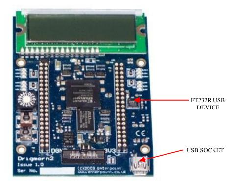
The USB interface on the Drigmorn2 is achieved using an FT232R USB to serial UART interface. The datasheet and drivers for this device are available from <a href="http://www.ftdichip.com">http://www.ftdichip.com</a>. When appropriate drivers are installed the Drigmorn2 USB port should be detected as a serial port. Alternative data optimised drivers are also available from FTDI.
