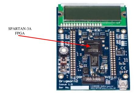
Drigmorn2 supports Spartan-3A devices in the FTG256 package. Drigmorn2 is normally available with commercial grade -2 speed devices fitted in the XC3S700A-4FTG256C size. For OEM customers we can offer a range of alternatives from XC3S400A to XC3S1400A as custom BOM variants.
