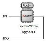
Right click on the icon representing the flash memory and choose program to load your program into the device. It is recommended that options to 'Verify' and 'Erase before programming' are chosen. Otherwise all defaults can be accepted. The programming operation will take some time (at least 3 or 4 minutes)
