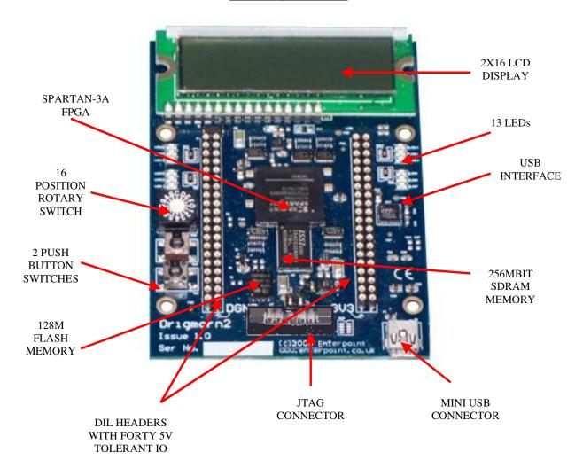
Your Drigmorn2 will be supplied un-programmed. Unless you have bought an OEM product your board will be supplied with either a Prog2 parallel port programming cable or a Prog3 USB port programming cable.
