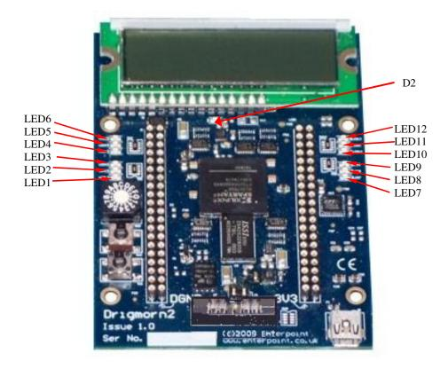
Drigmorn2 has 13 LEDs. There is a single red LED in the centre of the board just above the FPGA, and 12 LEDs arranged into 4 blocks of three, one of each block being red, orange and green. This is to enable users to simulate a traffic light sequence. The LEDS may turn on dimly when power is applied to the board. The relevant IO pin for an LED needs to be asserted high to ensure the specific LED turns on, and High impedance 'Z' to turn them off.
