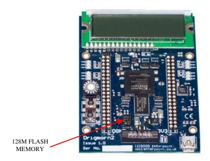
The M25P128 SPI flash memory device configures the FPGA when it is powered providing a suitable bitstream is programmed into the device. The M25P128 has a capacity of 128Mbits with a single configuration bitstream for Drigmorn2 taking 2.7Mbits (XC3S700A) . Any remaining space can be used for alternative configurations or code and data storage.
