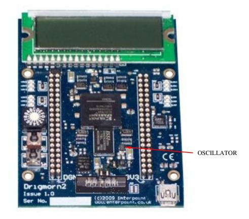
The main oscillator on the Drigmorn2 is an ASEM 25MHz oscillator. The oscillator is situated as shown and is connected to the FPGA on **PIN N9**, which is a global clock pin on the FPGA.
