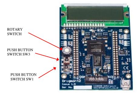
The Drigmorn2 has two push button switches and one 16 position hexadecimal rotary switch. To use these switches it is necessary to set the IO pins connected to the switches to have a pull up resistor in the FPGA. This is set in FPGA constraints file. Any switches pressed, or made, will then give a LOW signal at the FPGA, otherwise a HIGH is seen. The two push button switches are connected to the following IO pins.
