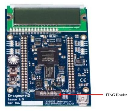
The programming of the FPGA and SPI Flash parts on Drigmorn2 is achieved using the JTAG interface. Principally it is anticipated that a JTAG connection will be used in conjunction with Xilinx ISE software. The free Webpack version of the Xilinx tools can be used to program the Drigmorn2.
