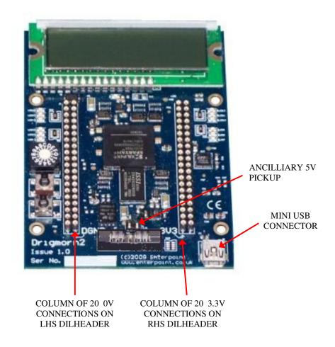
Drigmorn2 is powered from the USB connector. The board should be plugged via a cable into the USB socket of a PC, Laptop or USB hub. Some USB ports may not be able to supply greater than 100mA and either a powered USB hub or a mains wall brick is suggested for these cases.
