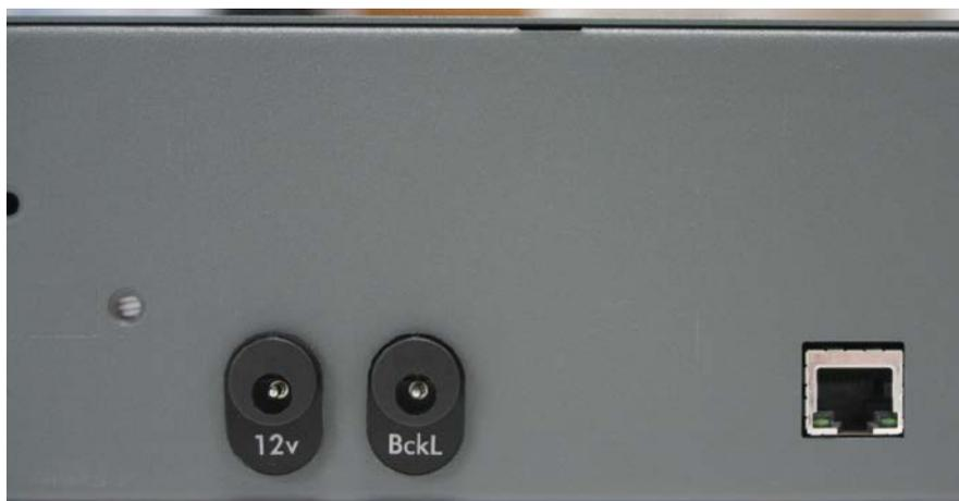
Both EFIS, CAP and FO must me also powered with 12V DC, plugged in the “Bckl” connector. If you have dimmer board, connect an output to the “Bckl” connector to manage it.
