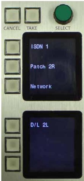
Pictured are the screens showing the normal operation of the **Route Select** mode.
