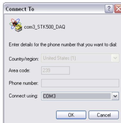
Figure 4.30 Screenshot of the Connect To window that HyperTerminal uses to establish at which COM port to receive or send data.
