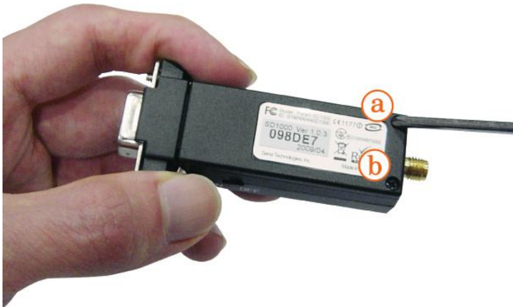
Figure 2-5 Remove Parani-SD1000 bottom cover
