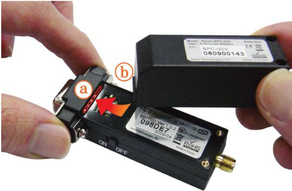
Figure 2-6 Attach the battery pack
