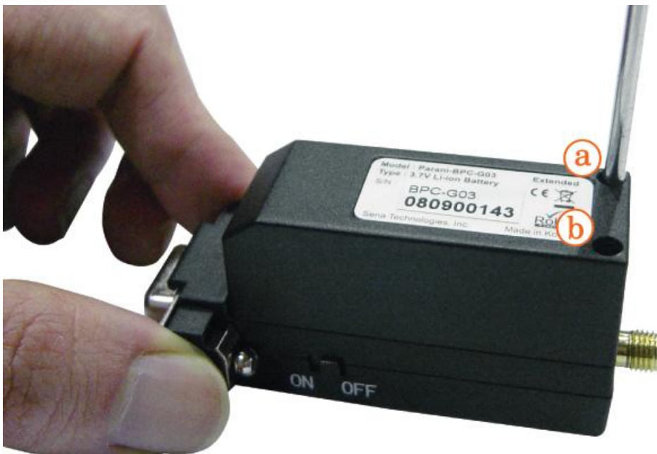
Figure 2-7 Fasten the battery pack
