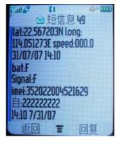
\*Tracking location, the SMS information about the lat./long. Received is the place received the GPS singal when the GPS singal is weak. Pls check the time received the SMS if there are some errors of the location.
